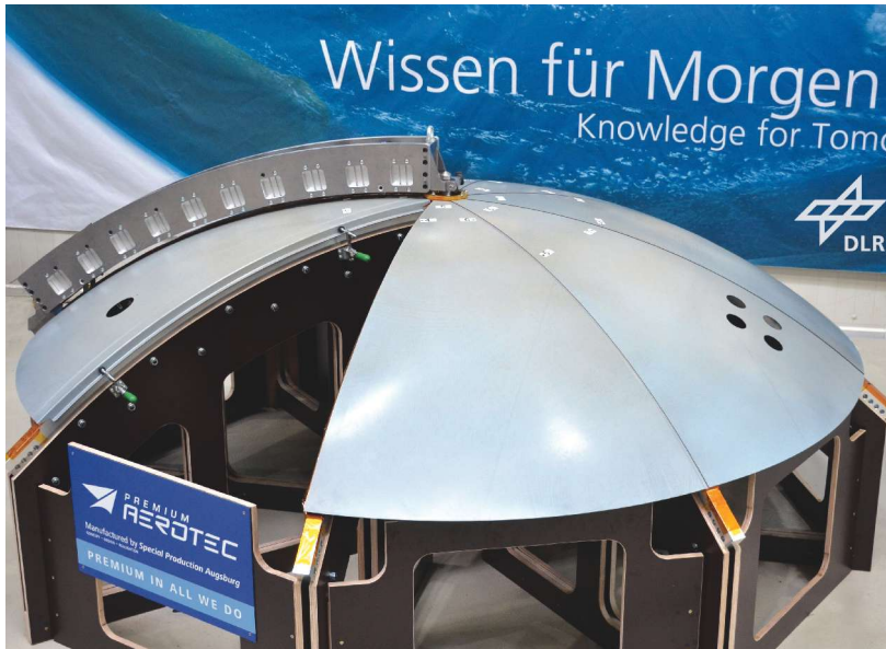
FIG. 2 CF resistance welding for rear pressure bulkhead
